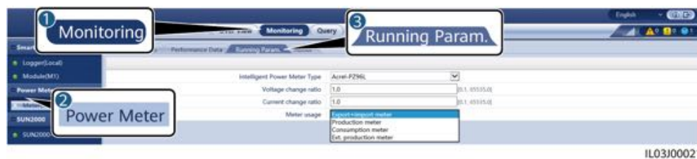
Figure 6-62 Setting power meter parameters
