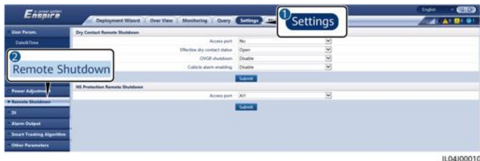
Figure 6-95 NS protection remote shutdown
