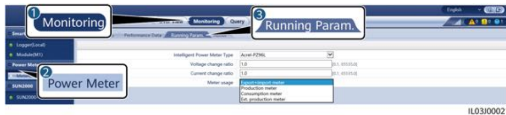
Figure 6-62 Setting power meter parameters
