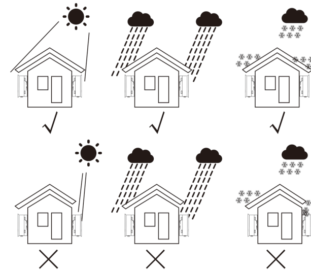
Figure 4.1 Recommended Installation locations
