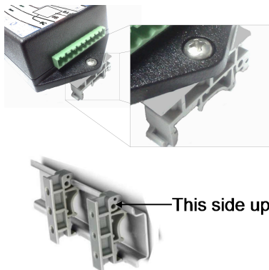
Figure 7: Mounting the meter on a DIN-rail
