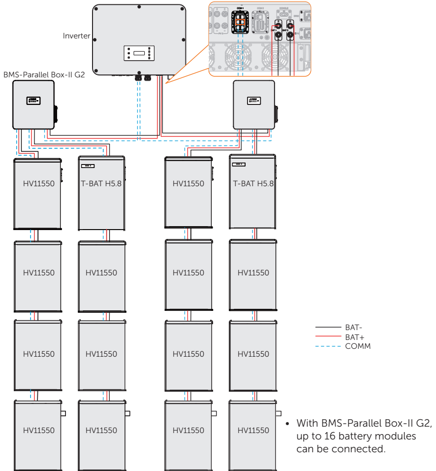
Figure 8-25 Battery connection with BMS-Parallel Box-II G2
