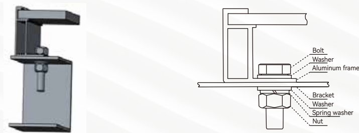
Figure 5 Bolt Installation of Mono-facial Modules
