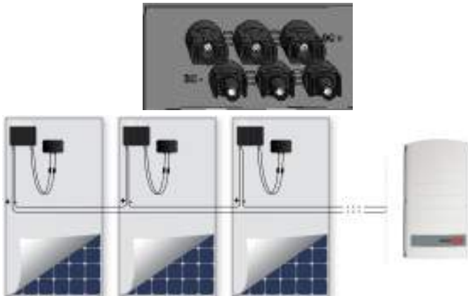
Figure 15: Inverter DC Connections
