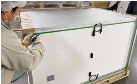
5. Remove internal straps and tapes. (recommend to work in pairs here)
