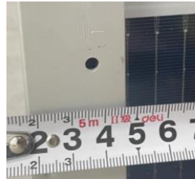
Fig. 8: detail view of equipotential bonding hole and symbol
