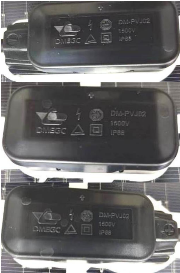
Fig. 5: detail view of closed junction box
